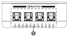
**1) OPTICAL OUT:** Connect to active speakers and or AV amplifiers with optical cable for audio output.
