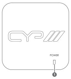
1 Power: This LED will illuminate when the unit is connected with power supply.
