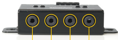
IR OUTPUT: 4 selectable ports Blaster or Emitter
